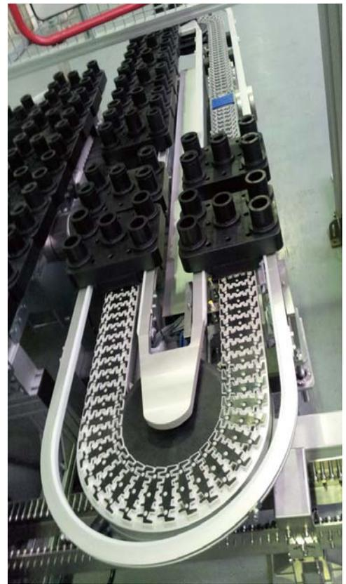
Conveyor with aluminum structure (for tooling pallet)
