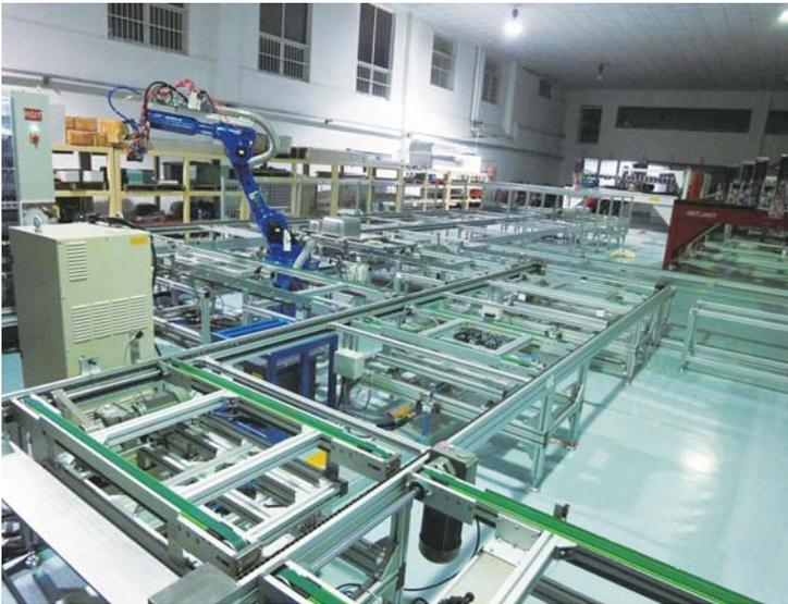
Automation assembly line (for rubber coating)
