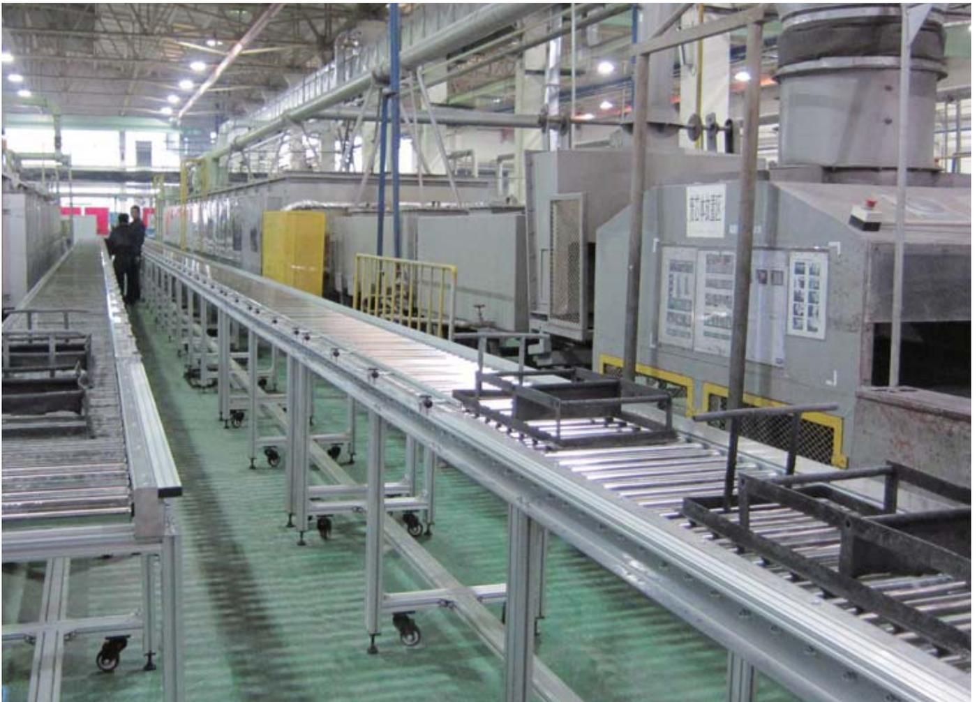
Carbon steel conveyor (for steel parts)
