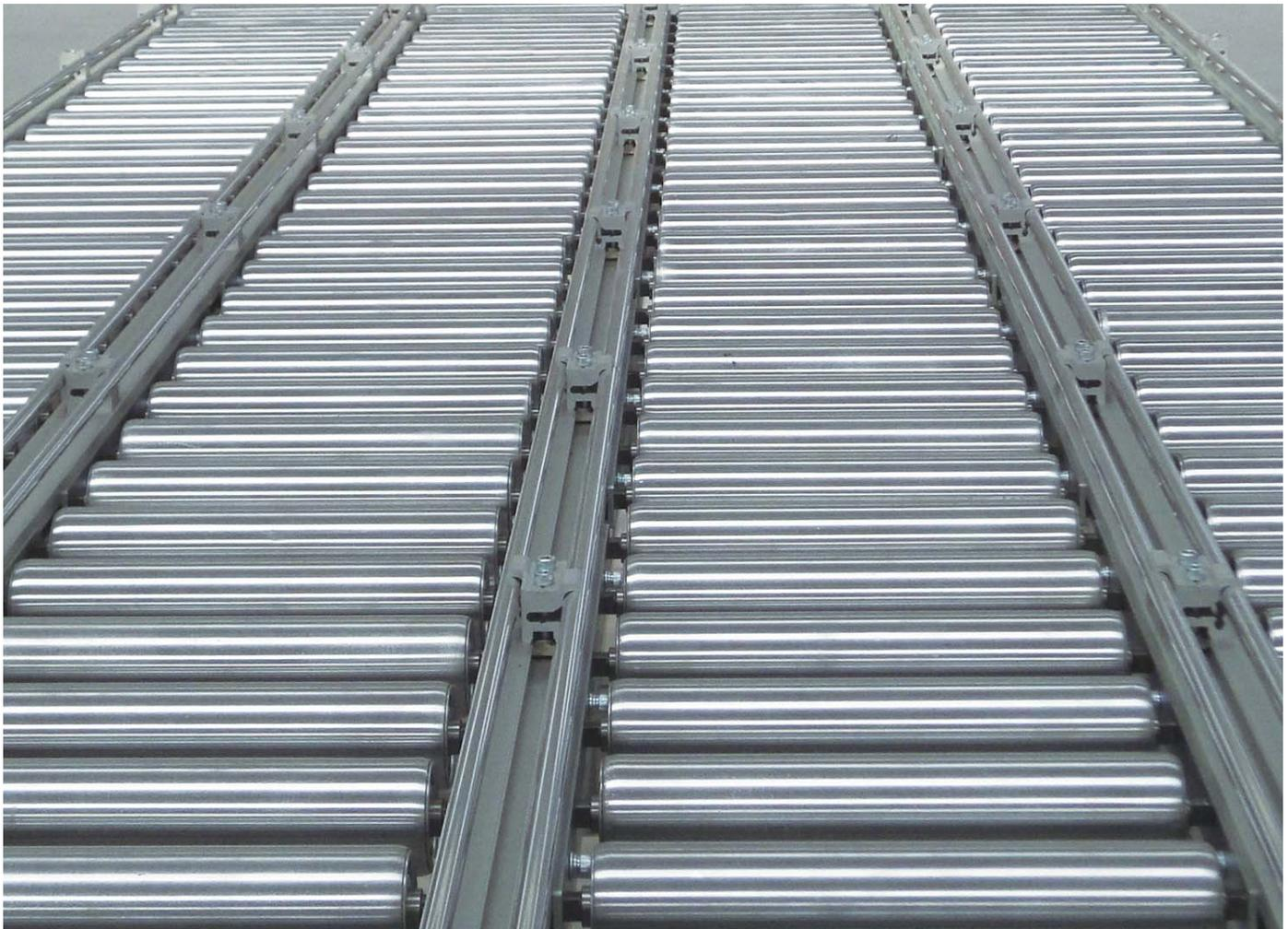
Zinc plated steel roller conveyor(automobile parts)
