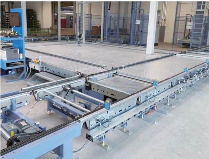
Heavy load capacity of chain conveyor (for 3000kg)
