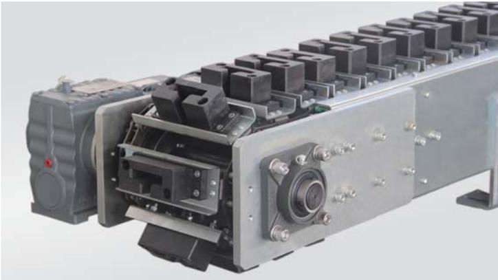
Chain conveyor with workpiece
